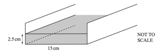
Water flows at a speed of 20 cm/s along a rectangular channel into a lake. The width of the channel is 15 cm.
